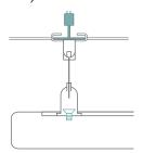
After acoustic panel is installed there will be a gap of 10 mm panel and wall.
